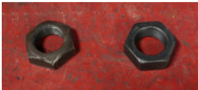
Old OE Nut (Left) vs. New MOOG Nut (Right)
